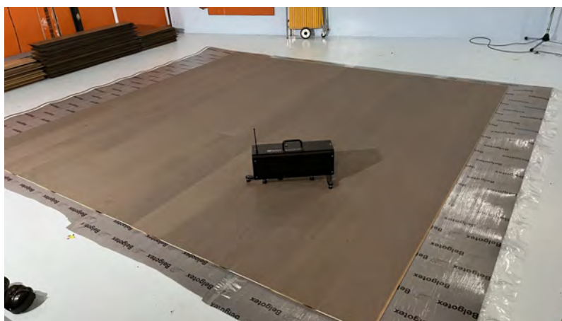
Figure 2.2: Parky 10mm finished floor system under test
